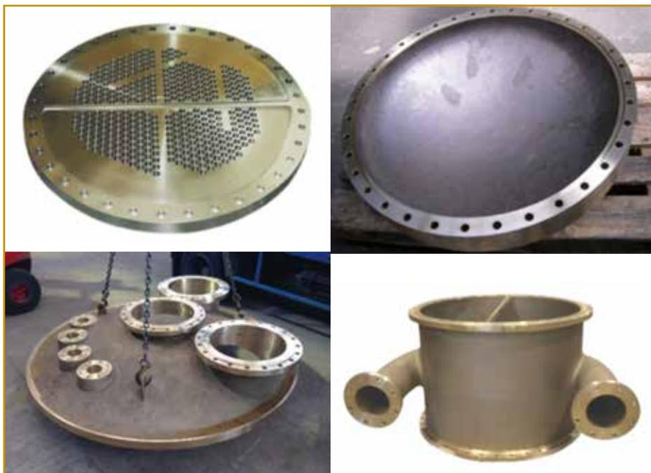
« Fig. 3. Examples of tube and shell heat exchanger parts, which can easily be cast in various aluminium bronze alloy grades . (a) ASTM B171 C63000 tube sheets. (b) ASTM B148 C95400 channels. (c) ASTM B148 C95800 float head. (d) Inoxyda 3P covers for chemical processes. (All photos courtesy of Inoxyda SA.)
