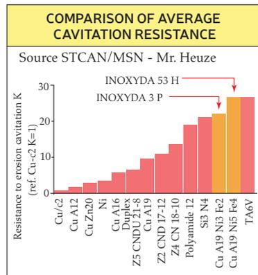
» Fig. 3. Resistance to cavitation (credit Inoxyda).
