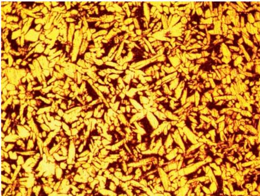
☞ Fig. 7. Micrography of casted aluminium bronze showing optimal structure to prevent dealuminization (credit Inoxyda).
