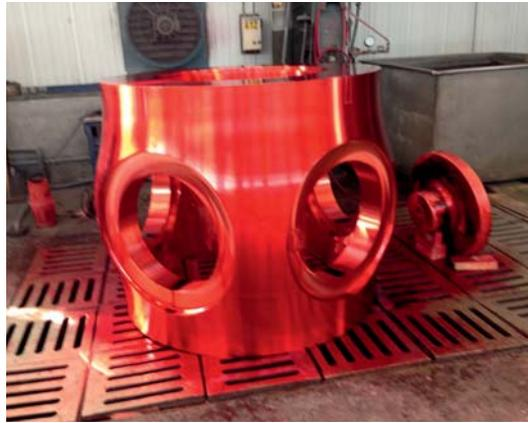
« Fig. 9. Dye penetrant test of pre-machined casting (credit Inoxyda).
