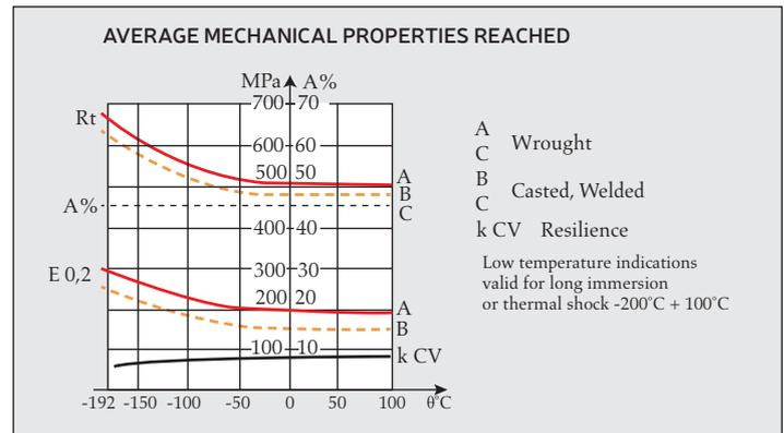
» Fig. 4. Effect of temperature on mechanical properties (credit Inoxyda).
