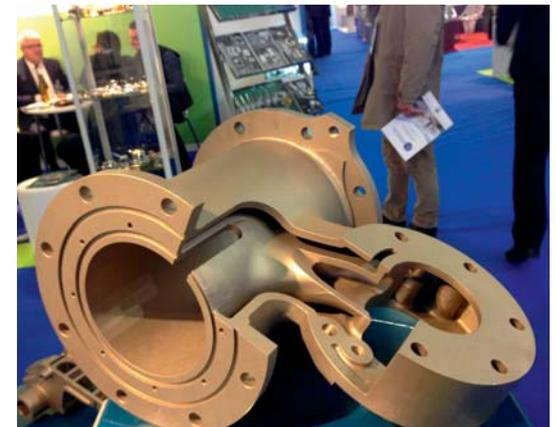
» Fig. 6. Valve casting using 3D printed cores (credit LBI Foundries).
