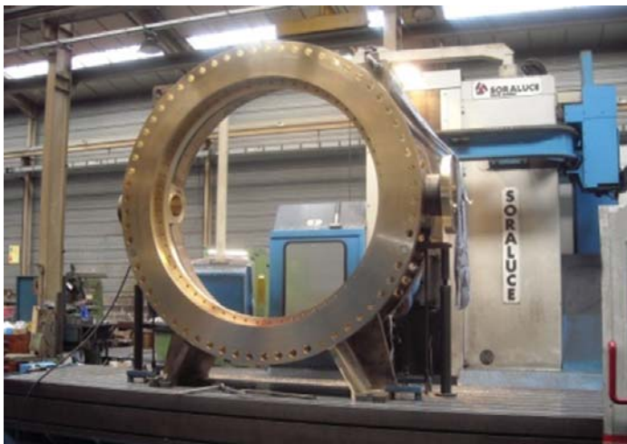
Figure 2: Valve body 2000mm dia 6000kgs. (Courtesy Inoxyda SA)
